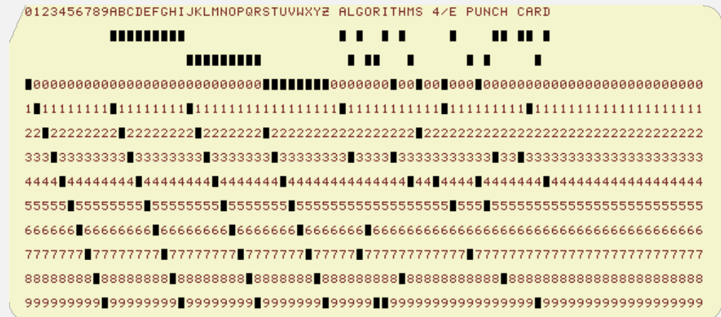
punch card (12 holes per column)
