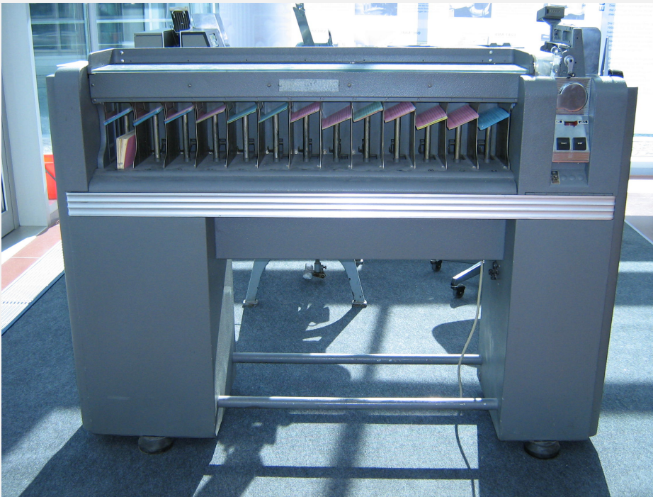
IBM 80 Series Card Sorter (650 cards per minute)
