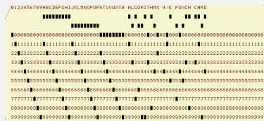
punch card (12 holes per column)
