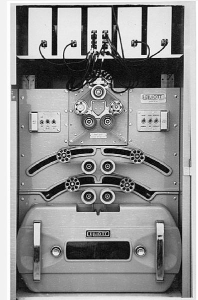
Elliott 405 magnetic disc (16K words)
