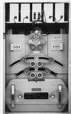
Elliott 405 magnetic disc (16K words)
