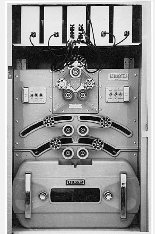
Elliott 405 magnetic disc (16K words)
