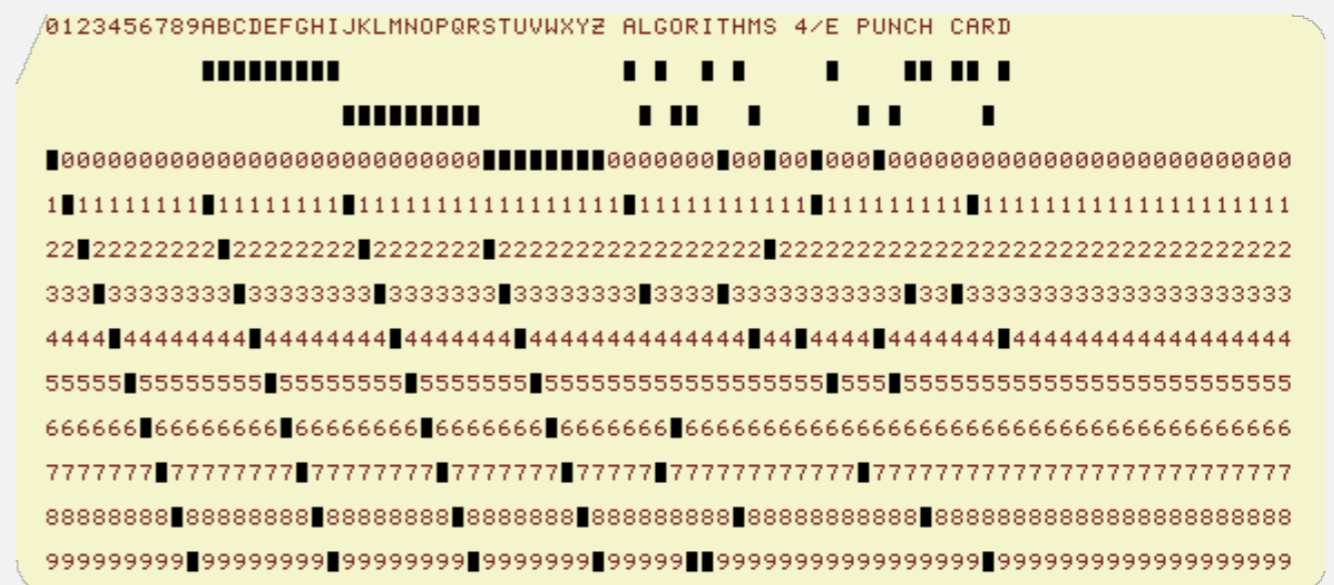
punch card (12 holes per column)
