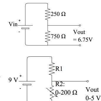
7. If your variable resistance sensor R2 ranges from 0–200 Ohms, and you'd like your Vout to be between 0 and 5 volts, what value should you choose for R1, in Ohms?
