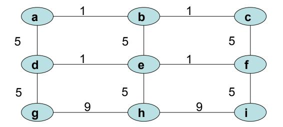
6d) Suppose the link f-e is overloaded with traffic. Identify a single weight change (on *just one link*) that would divert traffic from source f to destination d away from the f-e edge *without affecting the path between any other source-destination pairs*. Avoid any reliance on how routers choose between multiple paths with the same (smallest) cost.
