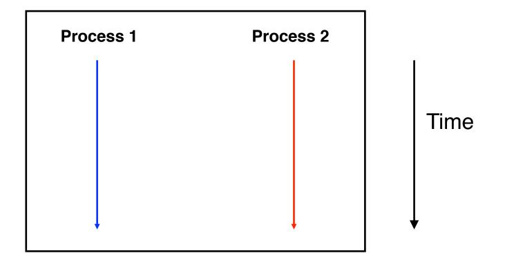
Hardware and OS give each application process the illusion that it is the only process running on the CPU
