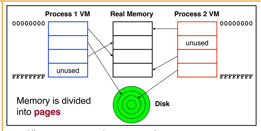
All processes use the same real memory Hardware and OS provide application pgms with a **virtual** view of memory, i.e. **virtual** memory (VM)
