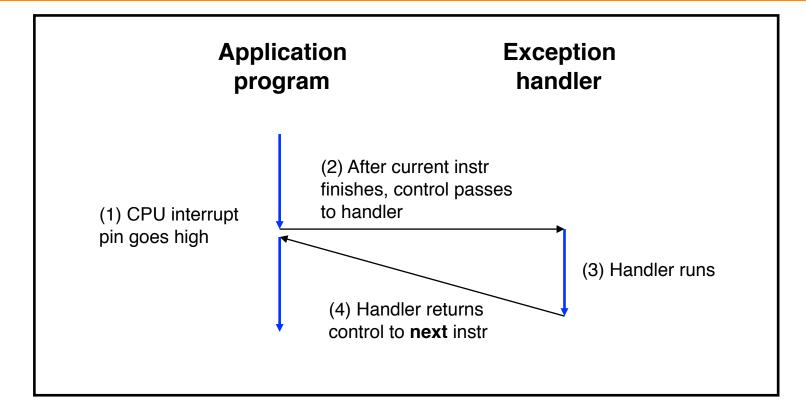
Cause: Signal from I/O device
