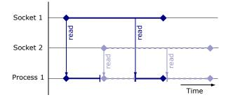
Objects are shown on the left side of the figure. Inter-object dependencies are shown as vertical arrows while intra-object dependencies are shown as horizontal lines. The start and end of an intra-object dependency interval is shown with a  $\blacklozenge$  symbol. Dependency intervals can be multiplexed over time as shown by the | symbol for Process 1. For this process, reading from different sockets starts the different intervals.
