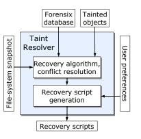
Figure 6: The Resolver architecture
