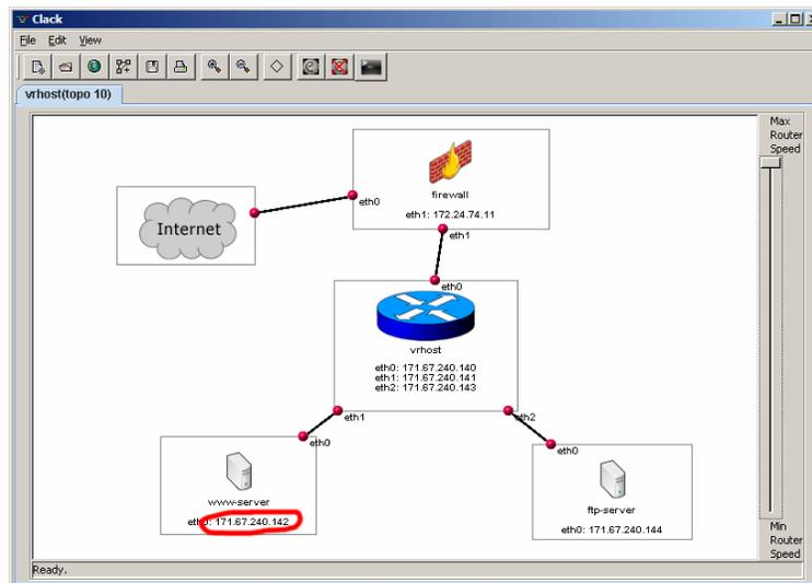
2. **You should see the Clack application window, as pictured above.** Clack is set up to simulate a small network consisting of two servers (www-server and ftp-server) connected to the Internet through a router (vrhost) and a firewall. In this picture, you and your lab mates exist in the cloud labeled “Internet.” We will refer to this picture as your *virtual world*.
