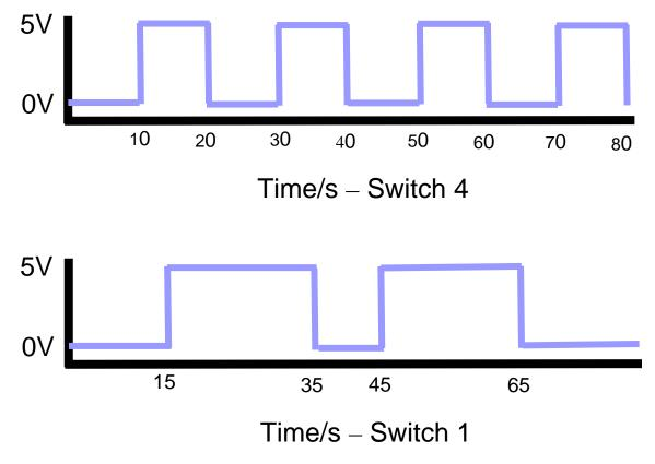
In your report, also describe what the output waveform would be if we had used the 'airlock' version of the D flip-flop? Recall that, in an 'airlock' flip-flop, the input is captured on the rising edge, but is only available on the output on the falling edge.
