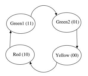
1. Fill in the state transition table of this FSM. The first row is filled out for you. CurrentState1 and CurrentState2 are the two bits of the current state. NextState1 and NextState2 are the two bits of the next state. The output bits are the signals that turn the three LEDs on/off.
