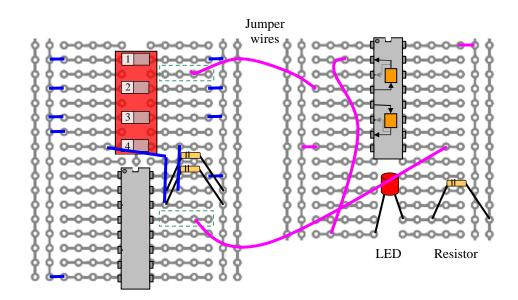
c. Connect the output of the D flip-flop to the LED.
