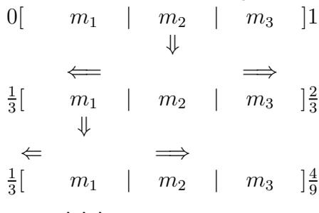
The above graph shows the encoding of message sequence  $\{m_2, m_1, \dots\}$ . We begin from the whole interval of  $[0, 1]$ . With the first message  $m_1$ , we split the interval proportionally according to the probabilities of the messages. Then we use the sub-interval corresponding to  $m_1$  as the current interval. With each consecutive messages, we repeat the above process to get smaller and smaller intervals. The final interval is the encoding for the whole message sequence.
