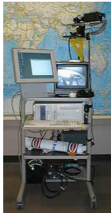
Fig. 6. The movable cart containing the necessary hardware to acquire range data (including power). The rangefinder and panning motor are in the upper right, there is a computer display and B/W monitor (for showing the laser position) in the center, underneath is a Dell PC, and at the bottom is a deep-cycle marine battery and power inverter.
