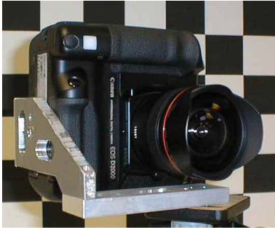
Fig. 7. The Canon EOS D2000 with mounting bracket to position the center-of-projection of the lens at the same location as the center-of-projection of the rangefinder. Since the light-sensor in this camera is smaller than film, it is necessary to use an extremely wide-angle lens for image collection. Here we show the 14mm lens, which acquires an image similar to a 24mm lens on 35mm film.
