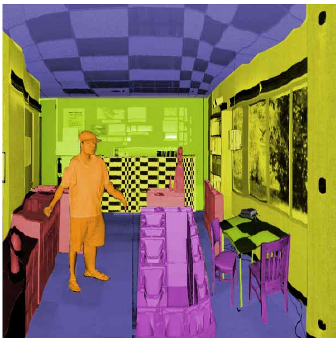
Fig. 16. Data collected while the scanning rangefinder was slowly pushed across the room. The position of the rangefinder is recorded when each column of data is collected. Note the irregular motion in the distorted ceiling tiles, walls and checkerboard patterns.
