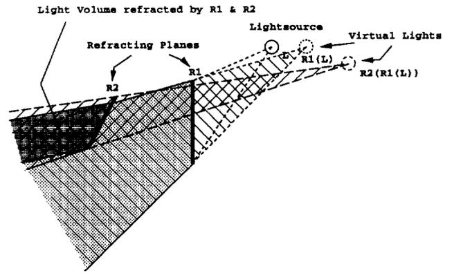
Figure 5: Light volume clipped by both refracting planes.
