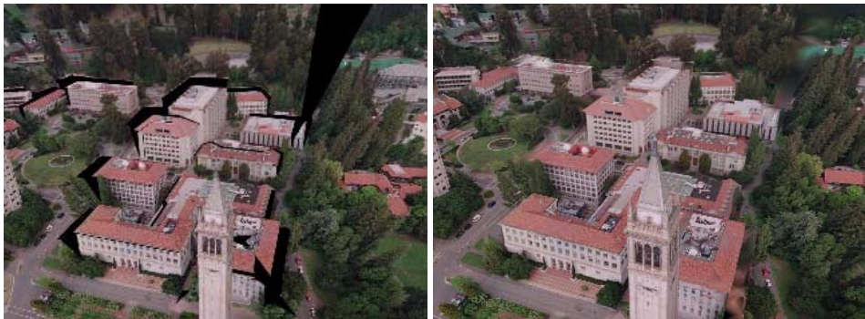
Fig. 4. The image on the left exhibits black regions which were invisible to all the original cameras but not to the current viewpoint. The image on the right shows the rendering result with all the holes filled. See also Fig. 8.
