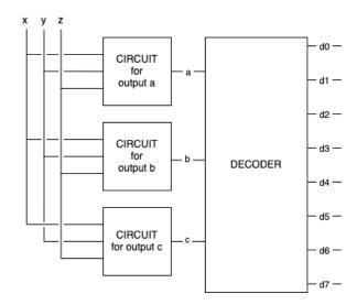
Of the decoder output lines d0, d1, d2, ..., d7, mark the ones that could possibly output a 1:
