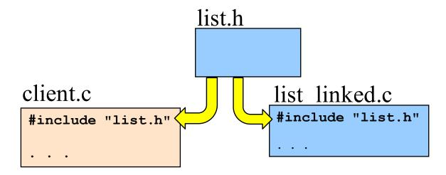
Arranging your ADTs and their clients in .c files like this, with the interface in .h files, is a *discipline* of programming, to enforce levels of abstraction, that you should use in C programming.
