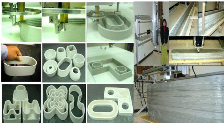
Fig. 2. CC in operation and representative 2.5D and 3D shapes and full scale concrete structures.
