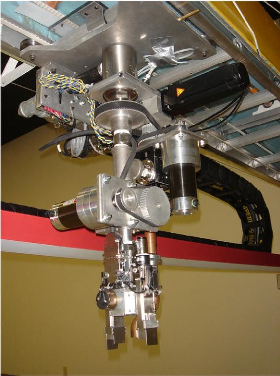
Fig. 8. Nozzle assembly and rotation mechanism.
