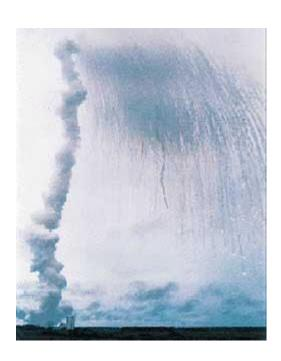
Ariane-5 self-destruction (1995) SW interface issue, backup failed Cost: \$400M payload
