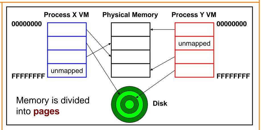
All processes use the same physical memory Hardware and OS provide application pgms with a **virtual** view of memory, i.e. **virtual memory (VM)**
