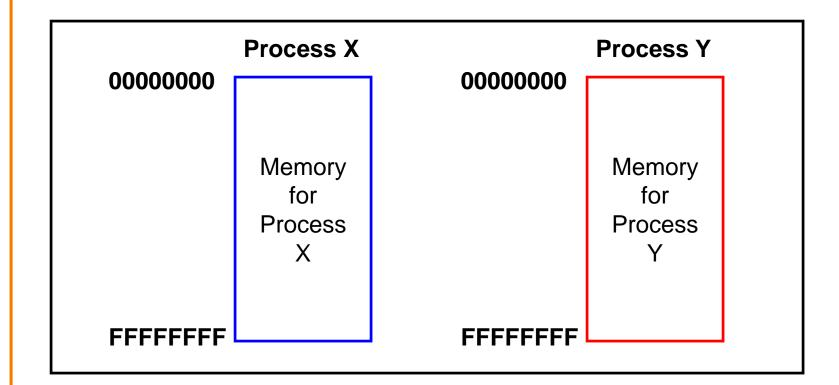
Hardware and OS give each application process the illusion that it is the only process using memory
