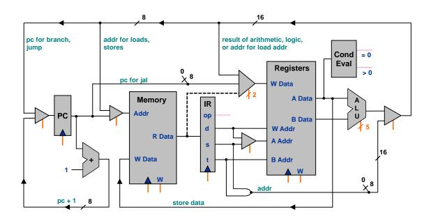
Suppose the dashed path were removed. For each of the opcodes below, would it still work even after the path was deleted? *Circle the correct answer on each line*. The **TOY reference card** is provided on the facing page.
