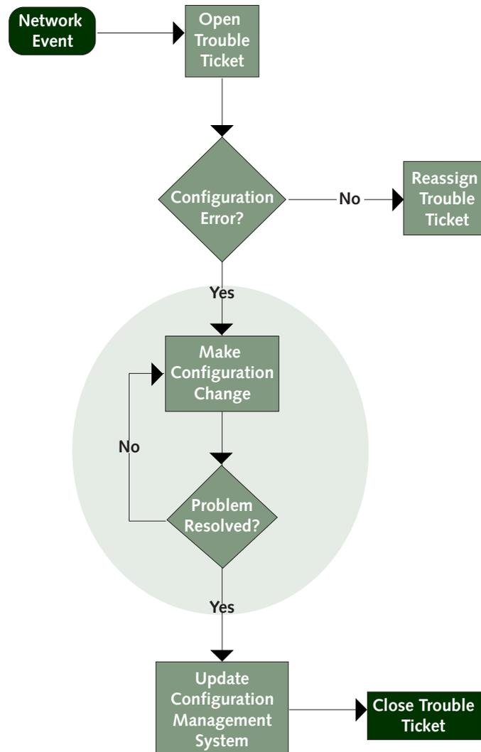
All of these problems lead to a higher cost of downtime, longer repair times and lower service reliability. The configuration of a device and the impact that configuration has on dependent devices is one of the first things a network manager will investigate during an outage. Without a consistent and controlled approach to device changes, it is nearly impossible to correlate those changes to network outages.
