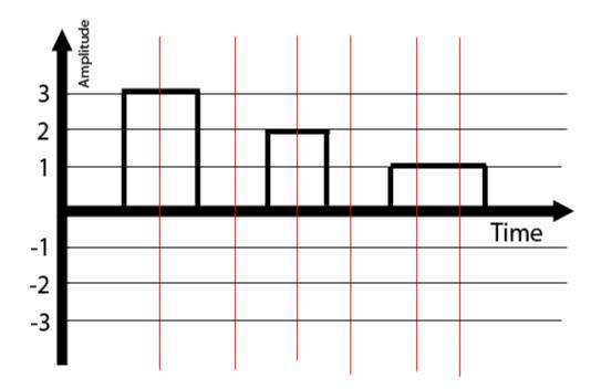
Assume that this square wave is being sampled at each moment in time that is marked with a vertical line. Label each sample with a 4-bit sequence (i.e. 0000) corresponding to the amplitude at that time.
