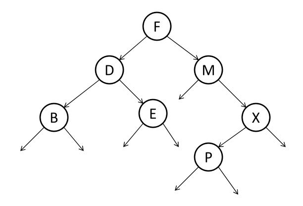
Binary tree: Each node x has a left child left(x) and a right child right(x), either or both of which can be null. Node x is the parent of both of its children: p(left(x)) = p(right(x)) = x.
