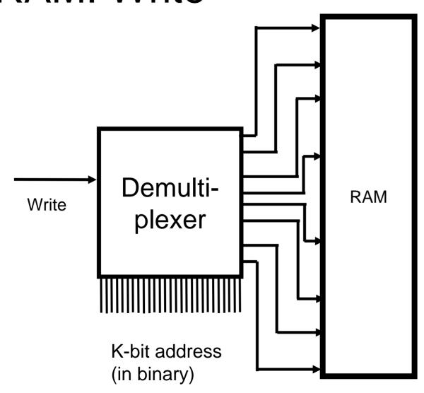
The k-bit address selects which of the 2<sup>K</sup> cells in the RAM gets its "Write" input toggled
