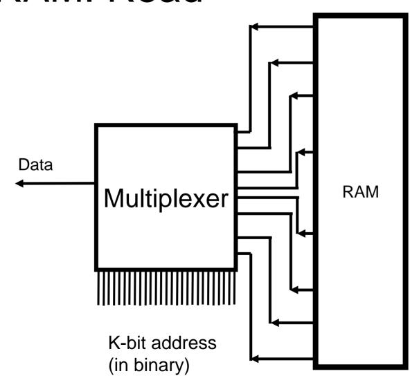
The multiplexer is connected to all 2<sup>K</sup> cells in the RAM; selects the appropriate cell based upon the K-bit address
