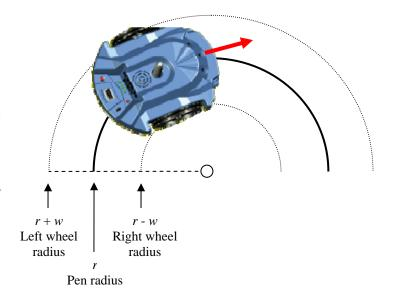
Measure w (half the distance between the wheels). Assume the left motor speed is 100% and solve the
