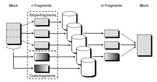
**Figure 3: Erasure coding example.** This example shows a 3-of-5 erasure encoding WRITE and then READ of a block. On WRITE, the original block is broken into three stripe-fragments and two code-fragments, then stored on five separate storage-nodes. On READ, any three fragments (stripe or code) can be retrieved from the storage-nodes to reconstruct the original block.
