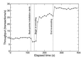
**Figure 7: In-place re-encoding of a live database system.** This graph shows the positive effect of re-encoding on the throughput that the TPC-C benchmark sees when accessing the underlying database. Ten trials are averaged and the standard deviation is less than 4 tps for each data point. Re-encoding changed the default block size of 64 kB to match the client's request size of 8 kB. The database was replicated on two storage-nodes and the re-encoding happened in-place.
