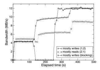
**Figure 6: Distribution change.** This graph shows the effect of migration and re-encoding as a function of the workload's read:write ratio. Each point is an average of ten trials. The standard deviation for each point was less than 0.5 MB/s. The back-pointer installation began at time 130, and the migration and re-encode began at time 140. The "blocking" case completed quickly but denied access to clients during the distribution change.
