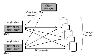
**Figure 2: Ursa Minor high-level architecture.** Clients use the storage system via the Ursa Minor client library. The metadata needed to access objects is retrieved from the object manager. Requests for data are then sent directly to storage-nodes.
