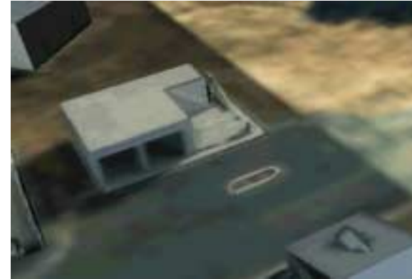
Model rendered from the pose of the helicopter sensor. Pose recovered after geo-registration process
