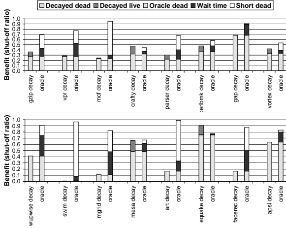
Figure 10. Lost opportunities for time-based decay (64Kcycle decay interval). SPECint2000 and SPECfp2000.
