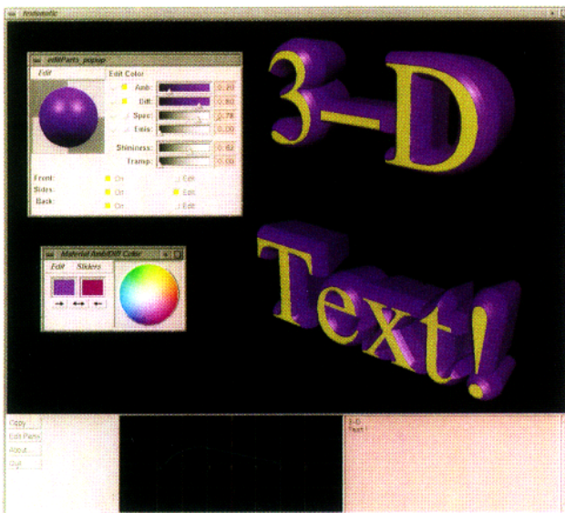
Figure 14. A three-dimensional text editing application. The small window at the bottom contains a profile curve manipulator which is used to extrude the 3D text.
