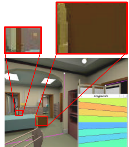
Plate 4. Images are rendered in parallel, one fragment per processor. a) Artifacts (highlighted in red) appear at the borders between fragments because of incorrect occlusion compatible traversal. b) Buffer zones between fragments are rendered during a second pass. c) Image rendered using two-pass traversal does not exhibit the artifacts of image (a).
