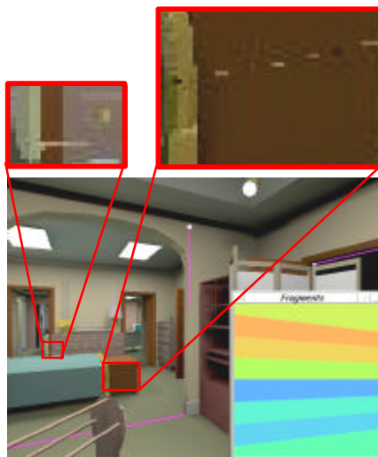
Plate 4. Images are rendered in parallel, one fragment per processor. a) Artifacts (highlighted in red) appear at the borders between fragments because of incorrect occlusion compatible traversal. b) Buffer zones between fragments are rendered during a second pass. c) Image rendered using two-pass traversal does not exhibit the artifacts of image (a).
