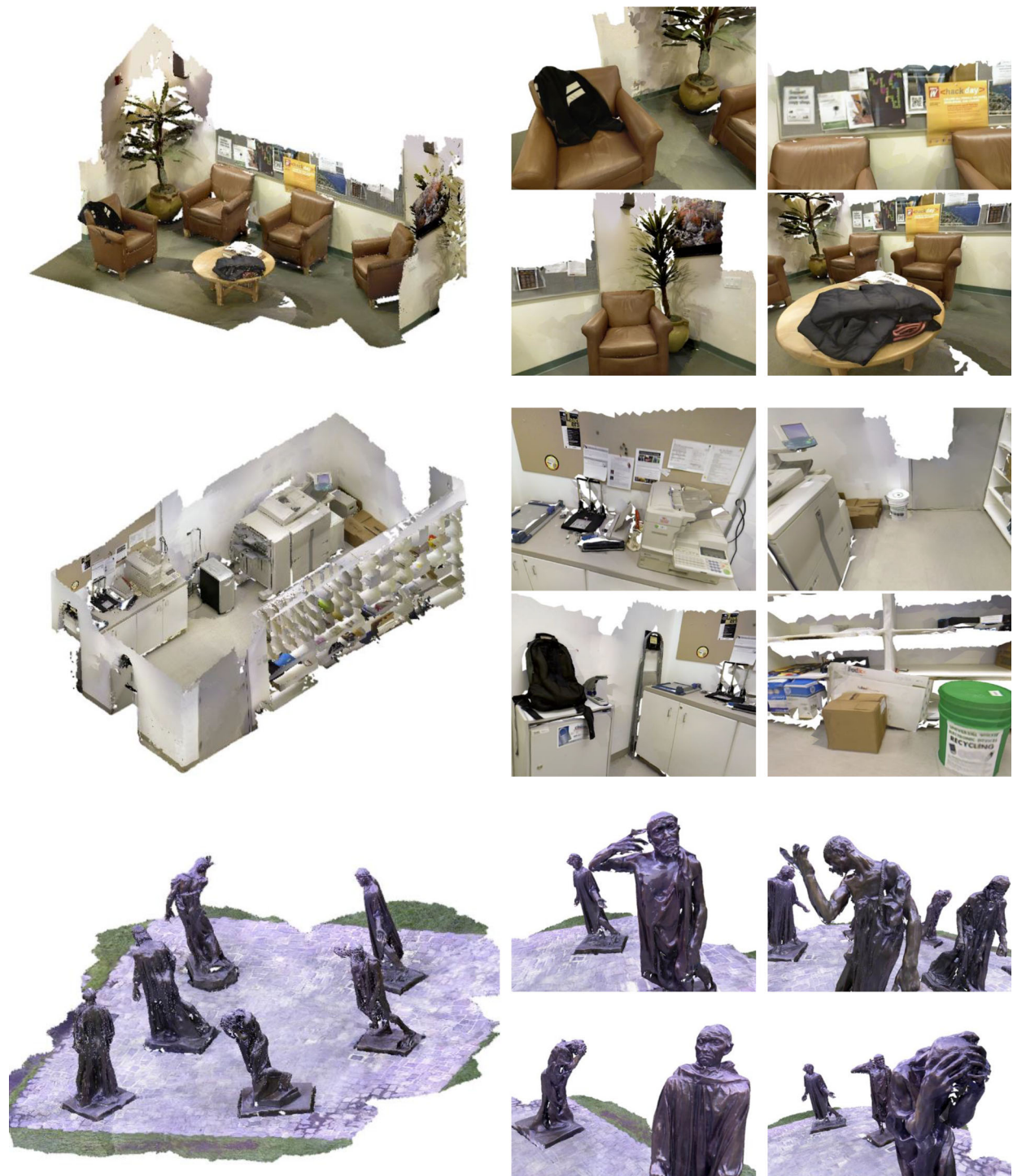
Fig. 12 Texture map generation and optimization results for large-scale 3D reconstructed models ( lounge, copyroom, burghers ). White holes in the rendering results have come from the missing geometry of the reconstructed models
