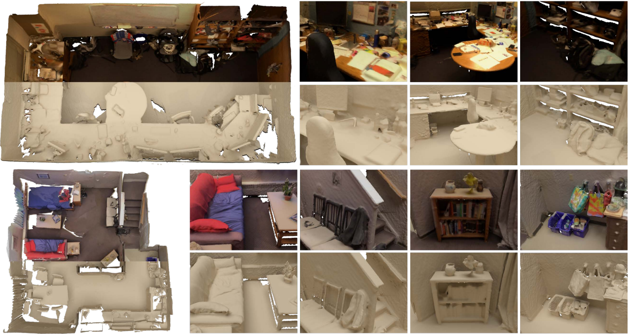
Fig. 3. Large-scale reconstruction results: our proposed real-time global pose optimization outperforms current state-of-the-art online reconstruction systems. The globally aligned 3D reconstructions are at a quality that was previously only attainable offline. Note the completeness of the scans, the global alignment without noticeable camera drift and the high local quality of the reconstructions in both geometry and texture. Scans comprise thousands of input frames, include revisiting and many loop closures.
