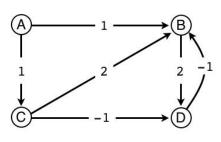
Bellman-Ford algorithm, for an implementation that starts with vertex A, proceeds in V phases, relaxing all of the edges in the graph in each phase. For the purpose of this question, to *relax* an edge is to check for evidence of a shorter path to its target than the best known so far, and a *successful relax* is one where a shorter path is found. The first phase is done for you.
