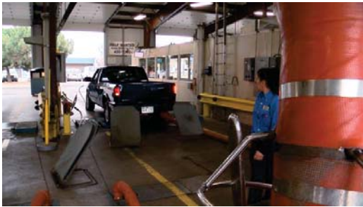
Traditional (since 1980s) DMV emissions testing
