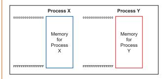
Hardware and OS give each application process the illusion that it is the only process using memory
