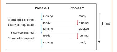
Throughout its lifetime a process's status switches between running, ready, and blocked
