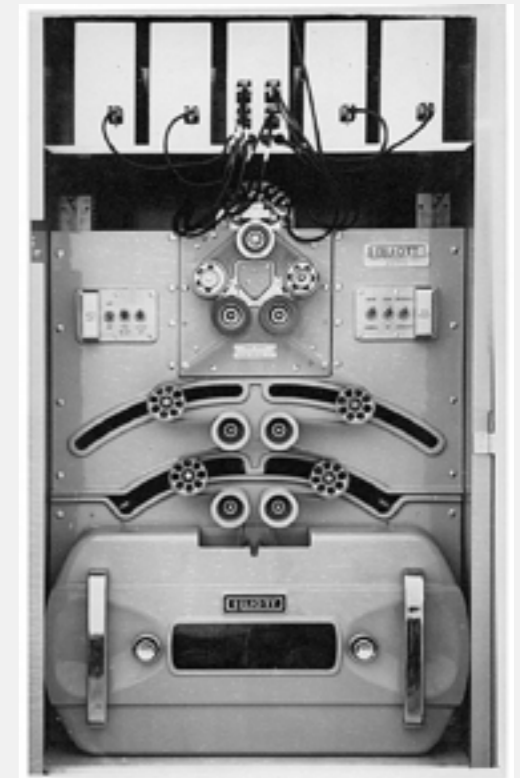
Elliott 405 magnetic disc (16K words)
