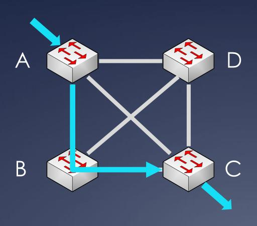
TE writes new value of routing state of B for tunneling traffic
