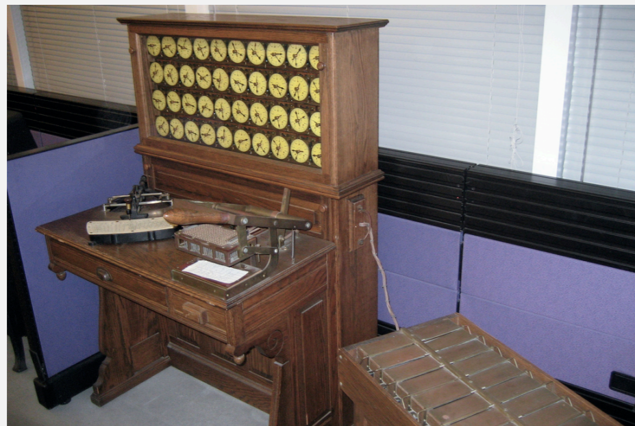
Hollerith tabulating machine and sorter
