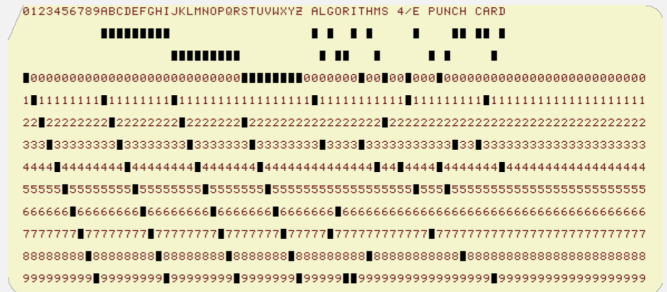
punch card (12 holes per column)
