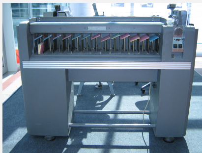
IBM 80 Series Card Sorter (650 cards per minute)
