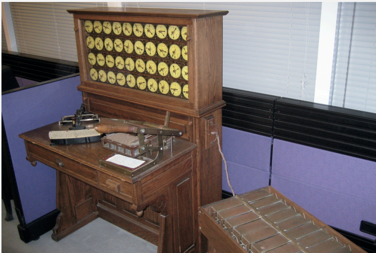
Hollerith tabulating machine and sorter
