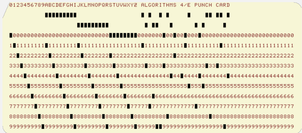
punch card (12 holes per column)
