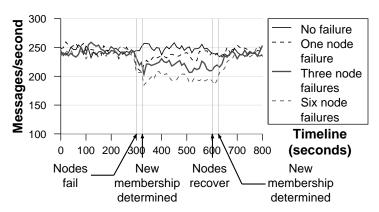
Figure 11. Reconfiguration timeline with replication.
