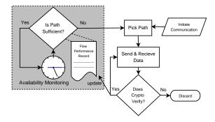
Figure 1: Control-flow of "availability monitoring" in ACR.
