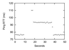
Figure 8: Observing OSPF route convergence (using ping)
