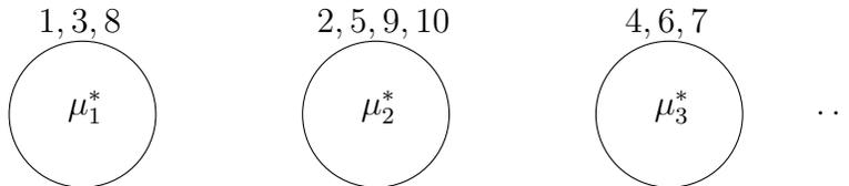
Figure 2: The Chinese restaurant process mixture. Each table  $k$  has a mean  $\mu_k^*$  and customers sitting at it are distributed according to that mean. Tables 1 through 3 and customers 1 through 10 are pictured.
