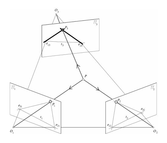
$$\begin{cases} \boldsymbol{p}_1^T \mathcal{E}_{12} \boldsymbol{p}_2 = 0 & \longrightarrow \\ \boldsymbol{p}_2^T \mathcal{E}_{23} \boldsymbol{p}_3 = 0 \\ \boldsymbol{p}_3^T \mathcal{E}_{31} \boldsymbol{p}_1 = 0 & \text{as the solution of linear equations.} \end{cases}$$
