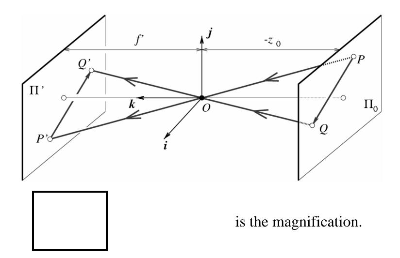
When the scene depth is small compared its distance from the Camera, *m* can be taken constant: weak perspective projection.
