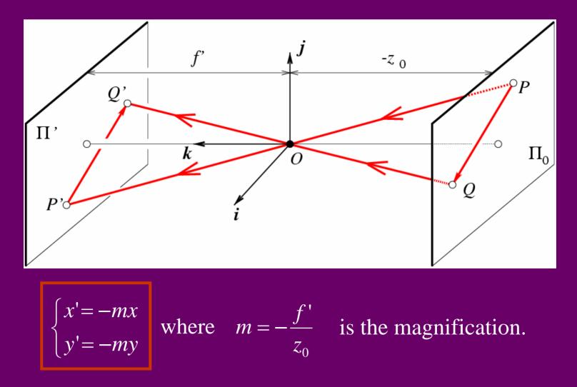
When the scene depth is small compared its distance from the Camera, *m* can be taken constant: weak perspective projection.
