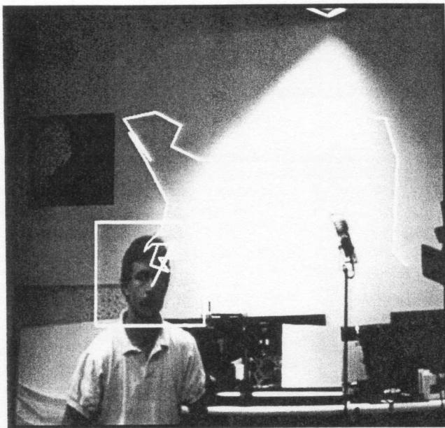
Figure 6. The head has been located—the image in the box is sent to the face recognition process. Also shown is the path of the head tracked over several previous frames.
